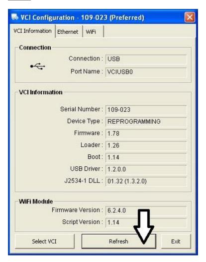
**Note:** VCI should now be connected in Adhoc mode. Each time the PC is booted up it will attempt to connect to the VCI wirelessly in Adhoc. No internet access is available while in Adhoc mode.
