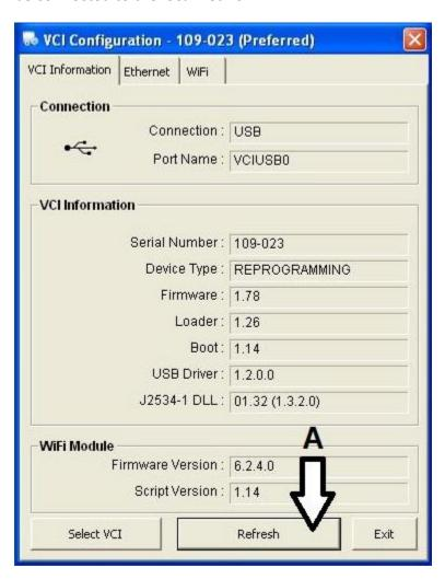
**B)** If it does not connect the first time, click the "OK" button on the error message and wait 30 seconds. Then select the "Refresh" button again. If it still does not connect, please contact technical support at 1-800-545-2220 ext. 1 for further assistance.
